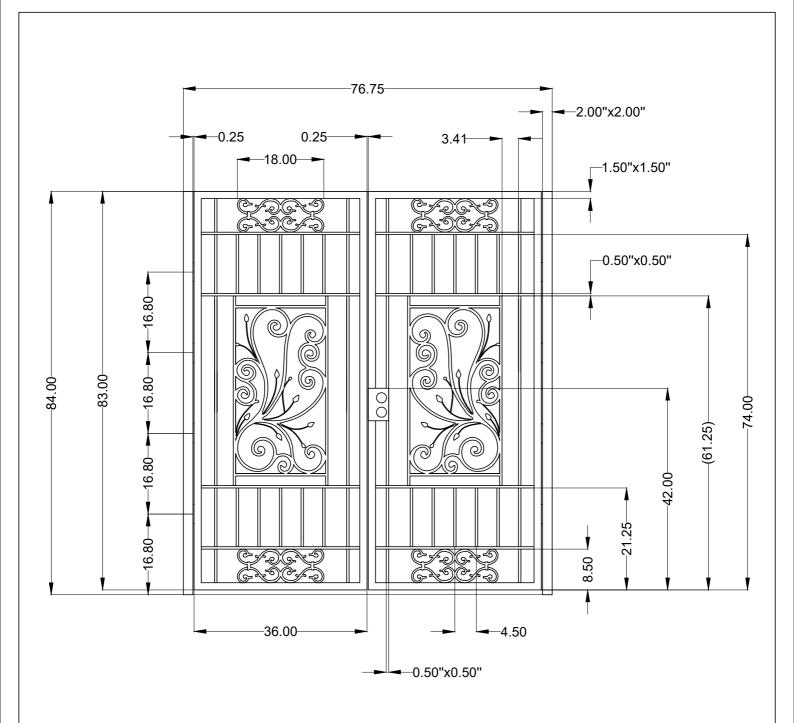
There are 7 pcs of pickets for each side of gate Frame =  $1"1/2 \times 1"1/2 - 14$  GA SQ. Steel Tube Pickets  $1/2" \times 1/2" - 16$  GA SQ. Steel Tube Steel pattern template dimension =  $39"1/2 \times 19"11/16$  Hinge =  $4" \times 4"$  Lock Box with H = 6"3/4, W = 4"1/4 and D = 1"5/16 Finish = Powder Coat
