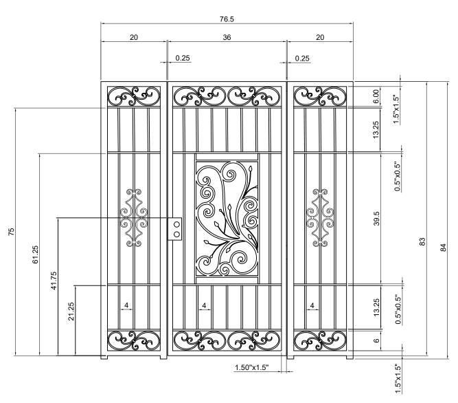
There are 7 pcs of pickets for each side of gate Frame=  $1"1/2 \times 1"1/2 - 14$  GA SQ. Steel Tube Pickets=  $1/2" \times 1/2" - 16$  GA SQ. Steel Tube
